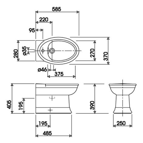
Please note: This bidet is not suitable for installation against blockwork walls due to pipework access restrictions.
